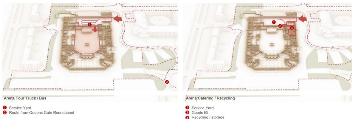
Figure 7: Access and servicing for the Arena
